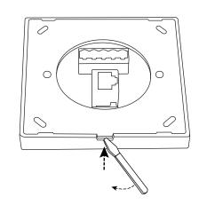
3.To put the back cover on the electrical box and fix it with the screw.
