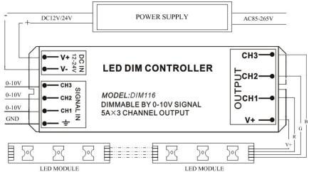
Remark: It can control various single color modules and RGB modules with the common anode.
