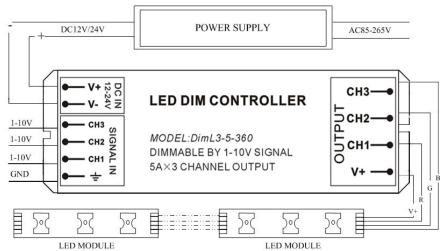
Remark: It can control various single color modules and RGB modules with the common anode.
