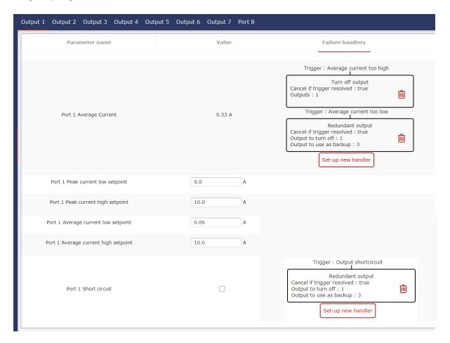
The action handlers have been set. When the MaNima Pollux measures a shortcircuit it will disable the output (1) and activate the secondary output (3).
