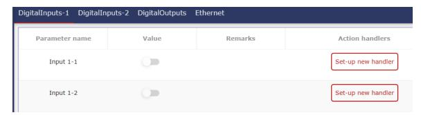
Using the action handlers it is possible to set trigger requirements for each Input, as shown in the table below:
