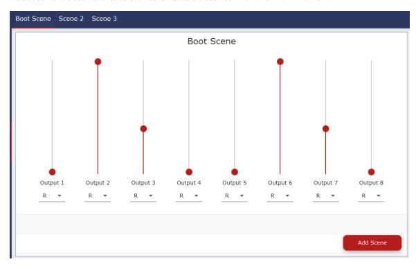
Use the sliders to adjust the output levels of each individual PWM port.
