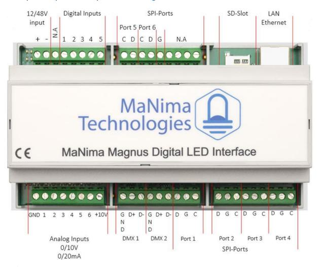
**12/48V input:** Connect 12-48VDC to this connector.
