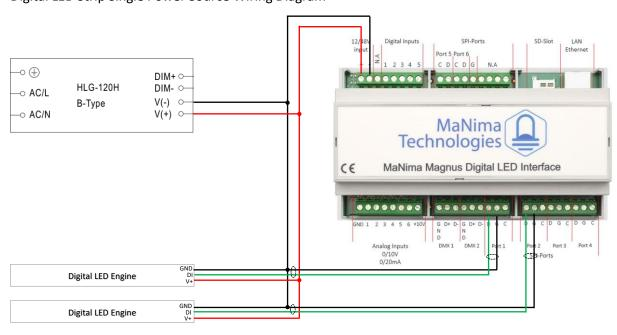
Digital LED Strip Multiple Power Sources Wiring Diagram
