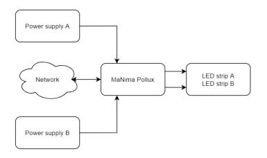
In this example, the LED strips are redundant placed inside a profile. Both are driven at about 50% to obtain sufficient lightning while keeping the temperature low.
