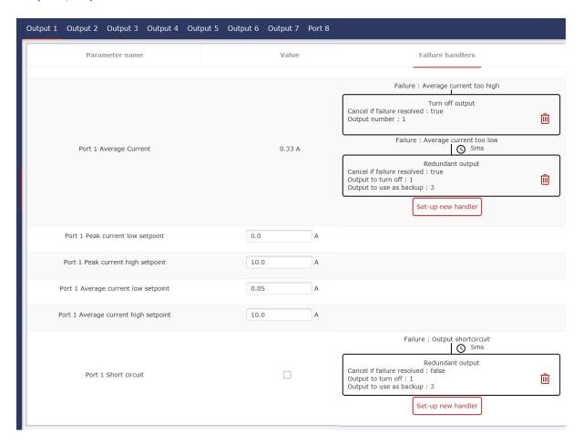
The failure handlers have been set. When the MaNima Pollux measures a shortcircuit it will disable the output (1) and activate the secondary output (3).
