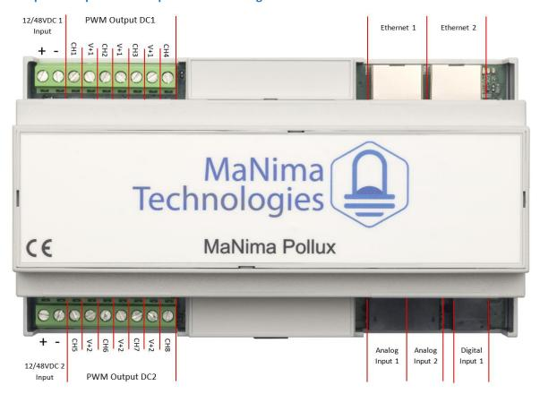
12/48V DC1: Power input for power source 1. Corresponds with 'DC1 PWM Outputs'.
