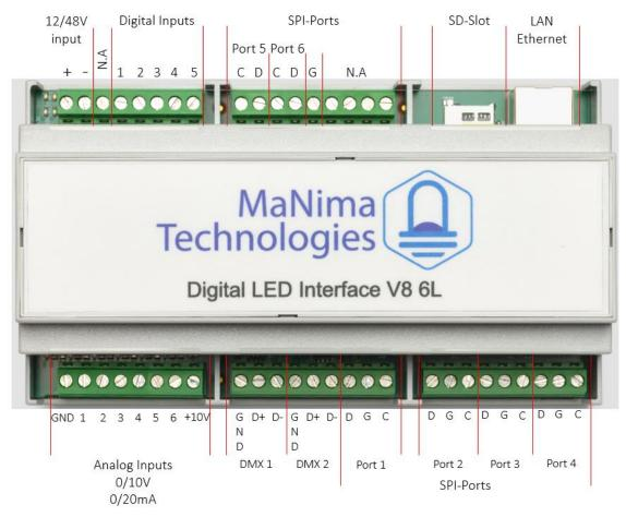
**12/48V Input:** Connect 12/48 Volts to this connector to power the MaNima Interface.
