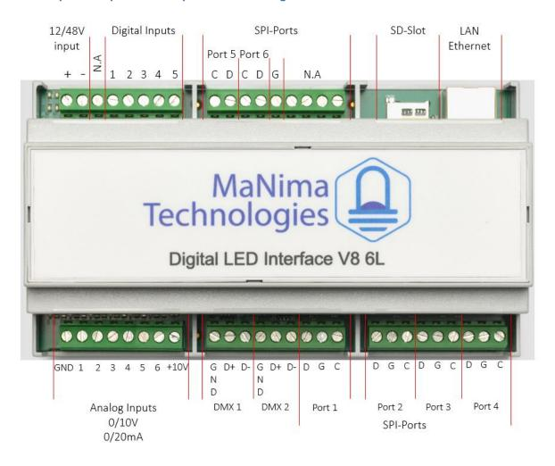
**12/48V Input:** Connect 12/48 Volts to this connector. DO NOT make short circuit while doing this, since it will seriously damage the MaNima LED Interface.
