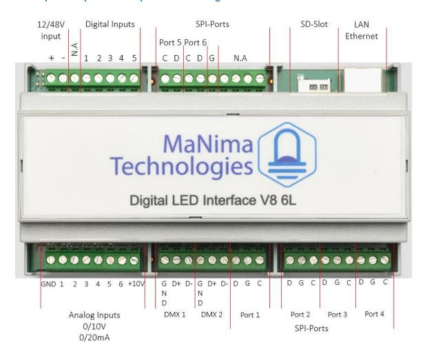
**12/48V Input:** Connect 12/48 Volts to this connector. DO NOT make short circuit while doing this, since it will seriously damage the MaNima LED Interface.
